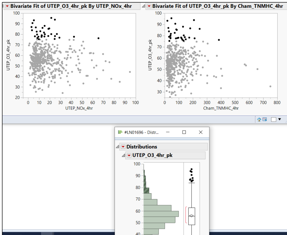
Figure 15 Comparison of NOx at UTEP and TNMHC at Chamizal morning averages and UTEP O3 averages using May – October // 2019 – 2021 data
