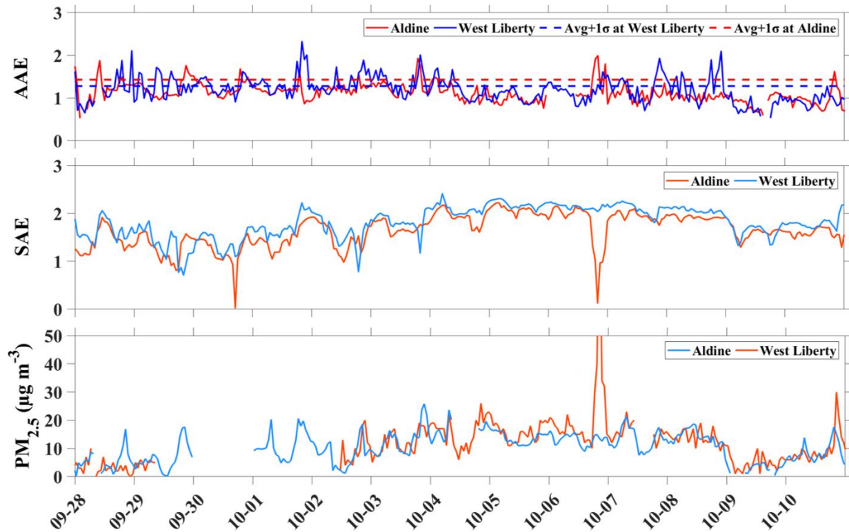
Figure 41. Time series (hourly average) of AAE and SAE values observed at West Liberty and Aldine sites during late September and early October 2020 at Houston.
