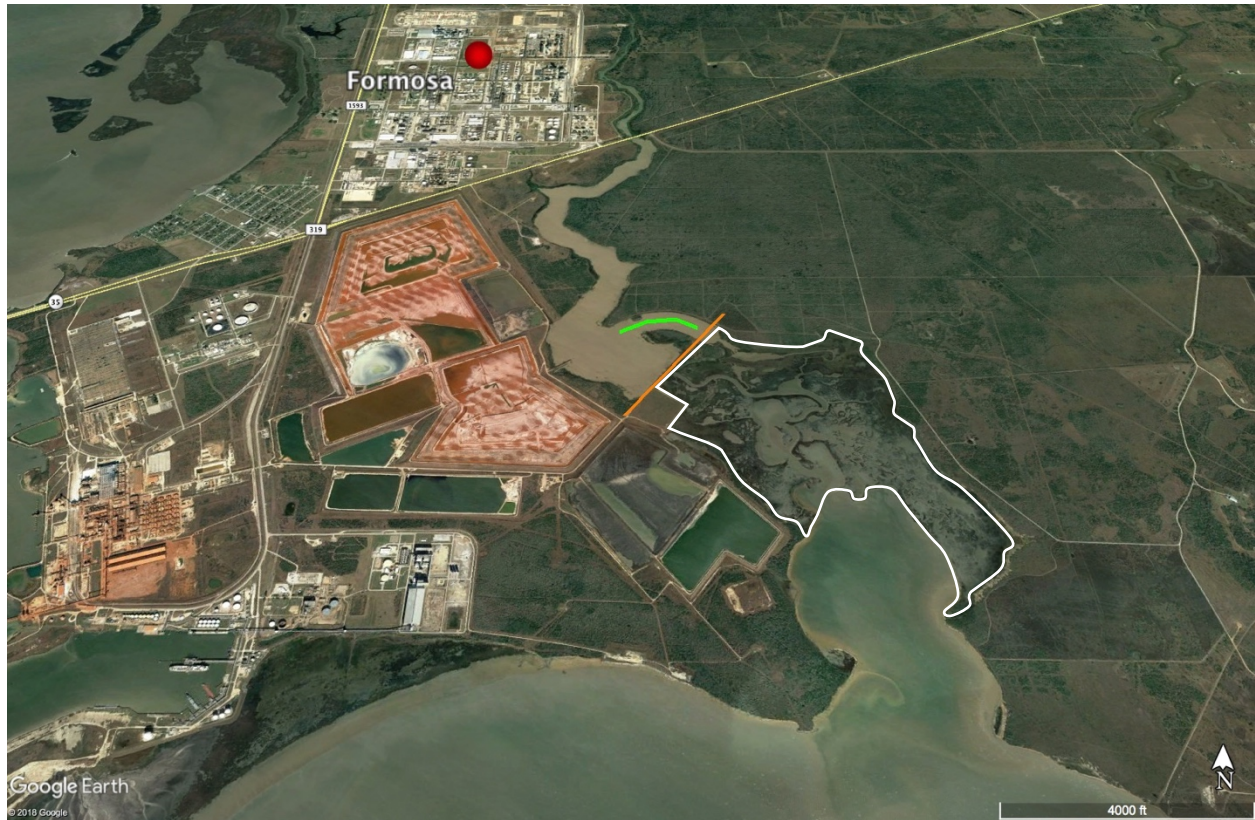
Figure 28. Cox Creek as it flows south of Formosa. The orange line is the constructed dam, the green line shows the spillway that allows excess water to flow into the downstream marsh and the white line delineates the boundary of the salt marsh.
